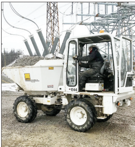
Reversibility enhances safety and eliminates the cost of another laborer to act as a spotter while backing up a rig.
