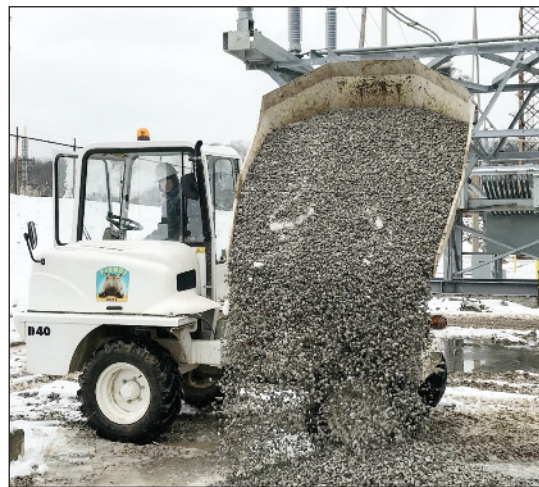
Features such as three-way dumping, directional reversibility and climate-controlled cabs make it easy for a site dumper to reach hard-to-access areas with obstructions.
